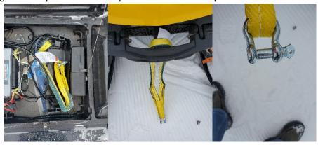
Never attach a tow rope or sling to the ski, as these are not designed lifting or tow points from the manufacturer.
